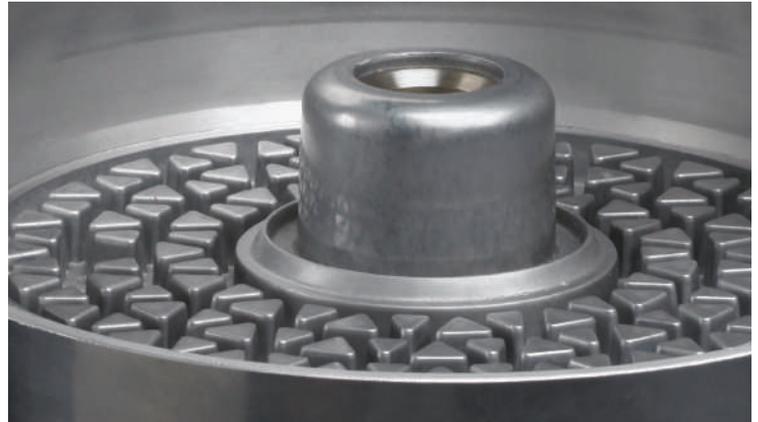
The intricately channeled base provides a large footprint to fully support the element under pressure, ensuring uniform loading of the element. Ultra-clean oil flows through the channels into the clean oil stream.
